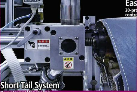
No water pool for cooling ST2 = Air cool/hot strand cutter 50 mm short tail, tubular cooling chamber
